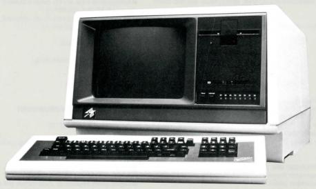
The UNISTAR™ 100 singleuser workstation is the first of a new family of powerful, 68000-based microcomputers that are designed and built to provide speed and versatility for the scientific, industrial and commercial markets. As a compact desktop system, the UNISTAR 100 combines cost effectiveness with high reliability to achieve the ultimate in individualized computing power for professional applications.
