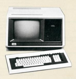
The CD100M is a compact desktop workstation which includes a versatile, intelligent terminal with advanced video features, a detachable keyboard, a Multibus\* card cage and a high-capacity switching power supply. Options include dual 51/4-inch, mini-floppy disk drives or one floppy and one mini-Winchester rigid drive.
