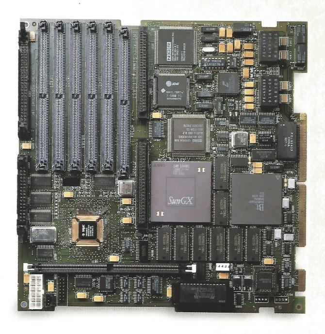
The RDI BriteLite LX utilizes the Sun SPARCengine LX board with the microSPARC CPU. This motherboard offers BriteLite users enhanced performance and functionality, as well as greater memory capacity. Bundled with an unmodified version of Solaris 1.1.1 or 2.3, the BriteLite LX ensures 100% compatibility with absolutely no compromises.
