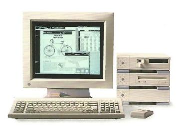
The SPARCstation ELC's five built-in ports provide connectivity to hard disks and tape and CD-ROM drives, plus the capability for multimedia and voice applications.
